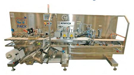
the flowpack machines. When convenient, the lug chain together with the product phasing system will be replaced by the individual smart carrier system. Able to load products on individual carriers moving independently and guided by potential differences on the magnetic field of the rail, this system is theoretically replacing any kind of product phasing system with advantages in terms of size and flexibility. The prototype machine will be presented in the current Interpack edition.
